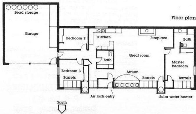
**Floor plan** emphasizes elongation of the south side of the building for good solar exposure. Rooms are laid out to aid natural heat flows. Note that the south collector/storage wall can "see" much of the north wall for effective distribution of heat.
