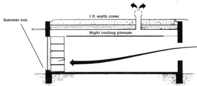
**Summer Mode** - Interior thermal mass is cooled down on summer nights by providing a natural air now path. Daily heat gains are rejected by this method through turbine roof ventilators. The cooled massive house is then closed up on hot summer days for comfortable living.
