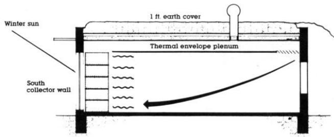
**Winter Mode** - Stored solar heat is released from the water containers as needed. Heat flows naturally by low temperature radiation and by warm air convection to the north side of the house, thus balancing comfort zones throughout the living space.
